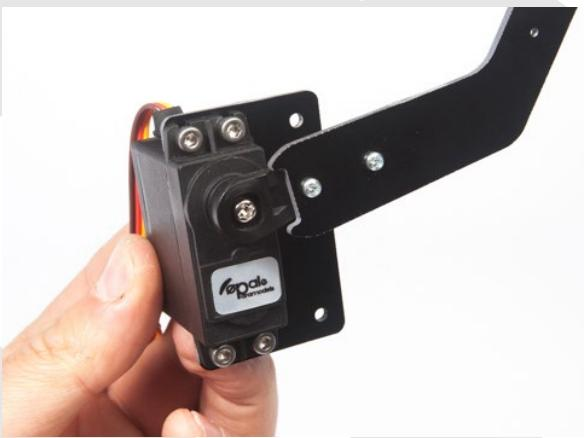
Position the whole thing as shown on the picture and tighten the whole thing with CHC M3-20 screws, washers and nuts.
