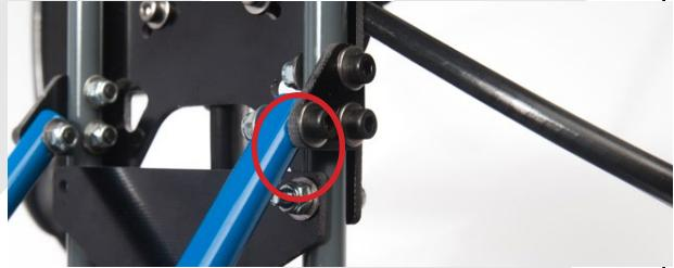
Use the ergots on the vertical plate to maintain the elastic. It will allow to hold the battery in the same position.
