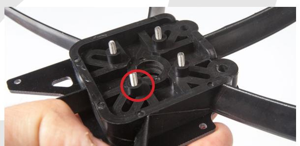
Mount the motor holder on the motor and then place the motor on the screws and tighten the motor with 4 x M3 nuts.
