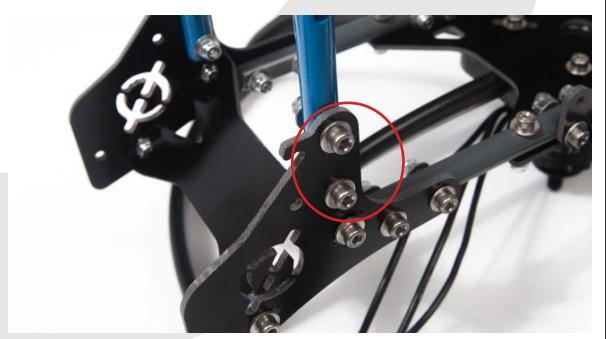
Then fix on this U steel part the other linking part with 2x CHC M3-16 screws, 4 washers and 2 nuts.
