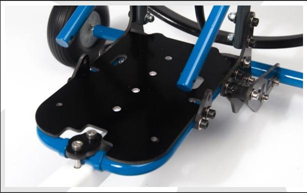
Then tighten once again the linking bar with the screws removed earlier. Careful though, the linking bar must be inserted in the plate hole.
