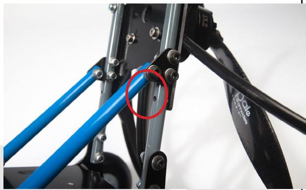
Insert the vertical plate of the kit. It has to slide between the horizontal plate and the X shaped plate at the back of the frame.
