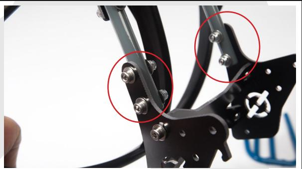
Place the U steel part and fix it on the previous part as shown on the picture with 4 x CHC M3-16 screws, washers and nuts.
